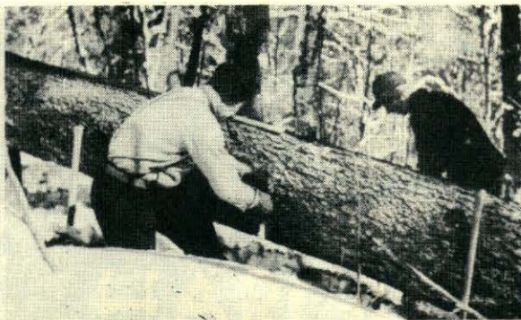
Spruce tree is bucked into sawlog lengths by loggers using cross-cut.
